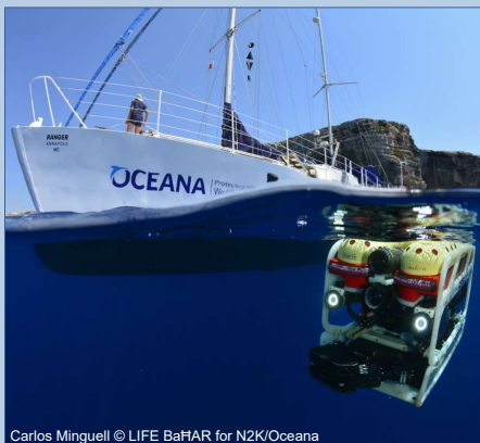
Figure 1. Saab Seaeeye Falcon DR Remotely Operated Vehicle being launched off the R/V 'Oceana Ranger' in the Maltese Islands.
